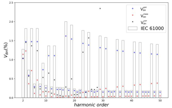
Fig. 6. Distortion of the background harmonic in the on the pre-connection procedure.
