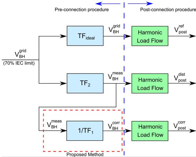
Fig. 2. Procedure to determine the harmonic distortion considering measurement on a CVT.
