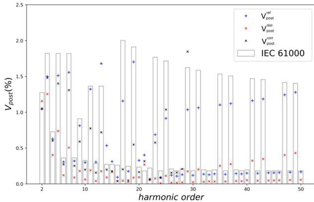
Fig. 7. Different harmonic distortion measurement on the post-connection procedure.
