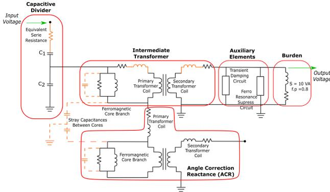
Fig. 4. Scheme of the CVT models.
