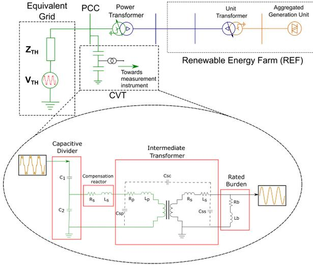
Fig. 1. CVT's elements and its location on the electric network.
